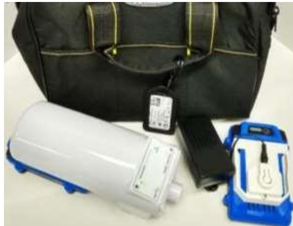
Figure 2: The ESU-110 is battery operated and is designed to be portable.
