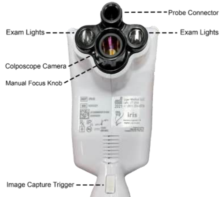
Figure 2: The IRIS is battery operated and is designed to be portable
